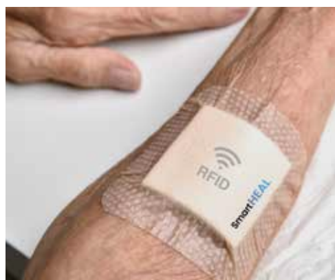
SmartHeal, Poland. A smart sensor for dressings which indicates how well a wound is healing by measuring its pH level.
