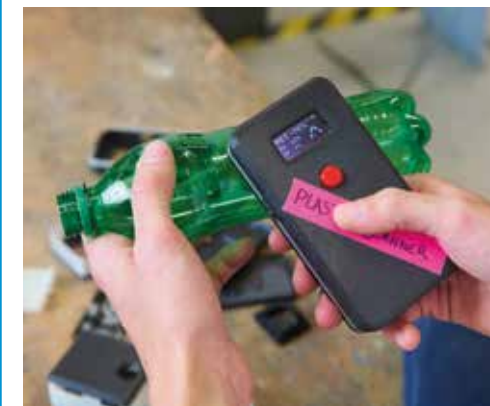
Plastic Scanner, Netherlands. A low-cost, handheld device to identify plastic for recycling.
