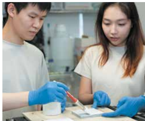
E-COATING, Hong Kong SAR. A sustainable, light-reflective paint that reduces the need for air conditioning.
