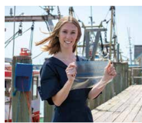
MarinaTex, UK. A home compostable alternative to plastic film, made from fish waste and red algae.
