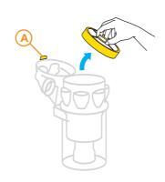
Lift filter release catch **A** and remove filter.
