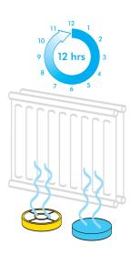
Dry for at least 12 hours. Ensure filter is completely dry before refitting onto the machine.
