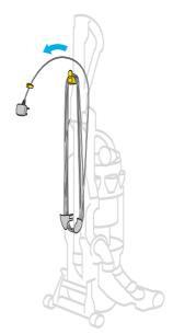
Wind cable anti-clockwise and secure with clip.
