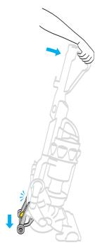
When finished, push the handle firmly beyond the upright position to drop stabilising wheels.
