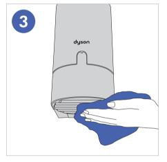
REGULARLY clean air inlets on base of motor bucket (under sink). Ensure plughole in sink is free from blockages so water can drain freely.
