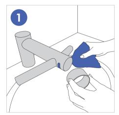
Wipe sensors using a soft cloth and non-abrasive cleaner then place cleaning cap over sensors to prevent activation.
