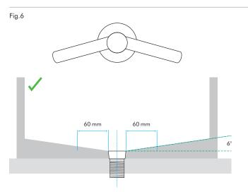
Minimum of 6° ramp angle from the edge of the drain hole of the sink will result in good drainage leading to reduced levels of splashback (minimum 60 mm radius).
