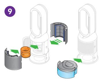
Push the evaporator back into your machine, making sure that it is securely in position.
