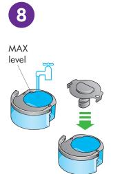
Refill the water tank to the Max level and wipe off any excess water and replace the cap, making sure that the cap clips are secured.
