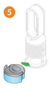
Slide the water tank into your machine until it clicks securely in place.
