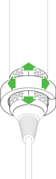
Slide the filter cleaning brush over the cable and onto the filter cage.
