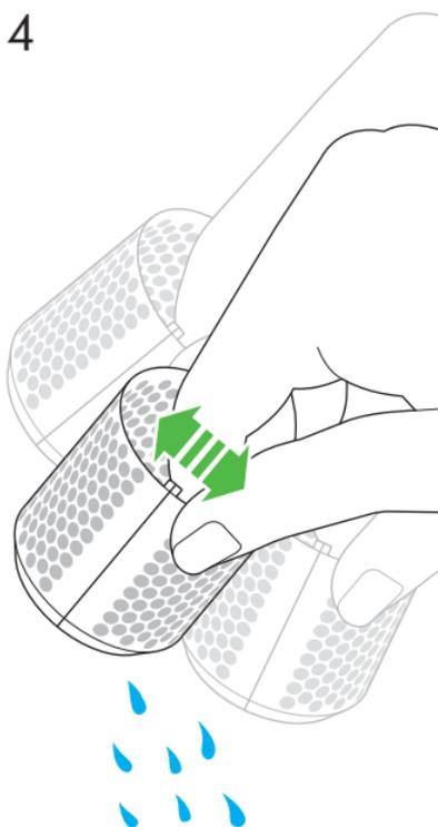
Shake the filter cage to remove the majority of the excess water, then leave to dry well naturally.
