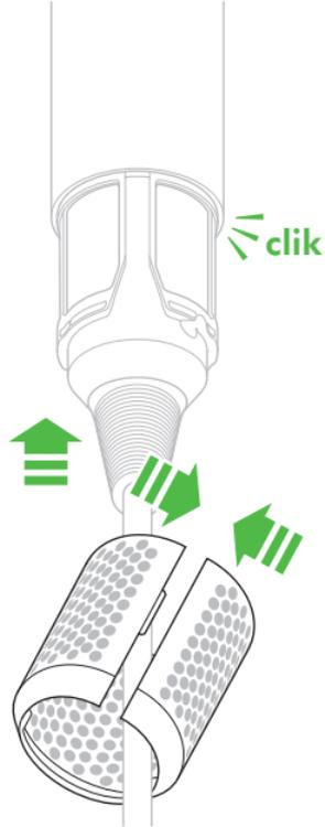
Gently pull the filter cage open and slide it onto the cable.
