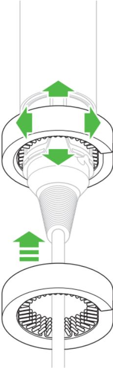
Using a rotating and up and down action, clean the filter mesh with the filter cleaning brush until all the debris has been removed.
