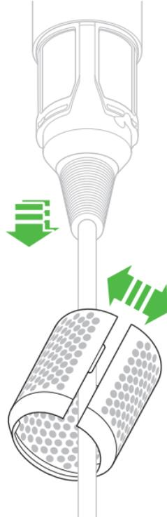
Hold the handle of your appliance and pull the filter cage downwards, onto the cable.
