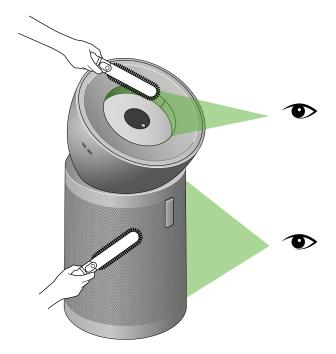
Eye icons identify where a user should regularly check for dust and debris, in outer cover and conic amplifier. Use a soft brush on the areas highlighted to clean the purifier.
