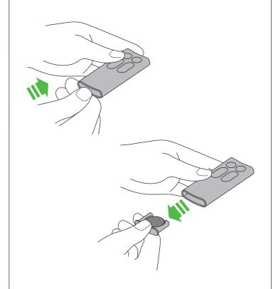
Press the end of the remote to release the battery.
