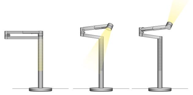
You can easily change the position of your light by independently rotating the optical head, arm and stem up to  $360^{\circ}$ .
