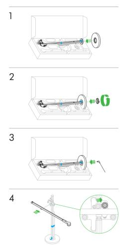
It is important that the light is assembled in the box as shown.
