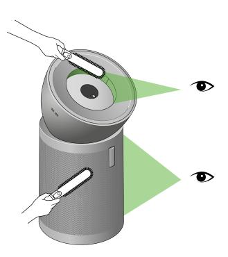
Eye icons identify where a user should regularly check for dust and debris, in outer cover and conic amplifier. Use a soft brush on the areas highlighted to clean the purifier.
