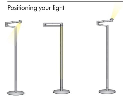
You can easily change the position of your light by independently rotating the optical head, arm and stem up to 360°.
