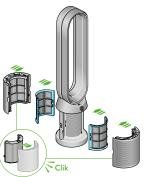
The air purifier fan with the filter covers open showing a HEPA plus carbon filter located in the filter covers and a catalytic filter. Arrows demonstrate that the catalytic filter is fitted directly to the base of the machine and the filter covers will need to be assembled onto the base of the machine.
