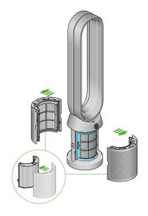
The air purifier fan with the filter covers open showing a HEPA filter located in the filter covers and a carbon filter. Arrows demonstrate that the carbon filter is fitted directly to the base of the machine and the filter covers will need to be assembled onto the base of the machine.
