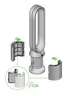
The air purifier fan with the filter covers open showing a 2 in 1 HEPA+ Carbon filter located in the filter covers. Arrows demonstrate that the filter covers will need to be assembled onto the base of the machine.
