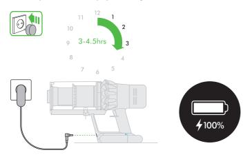
Connect to the charger either directly or in the docking station.
