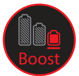
The screen showing the machine set to Boost mode with a red battery to show that this will give the shortest battery life of the three modes.
