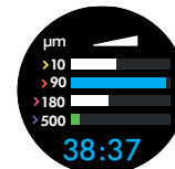
The screen, on the end of the main body, showing a graph of the sizing and counting of the dust particles.
